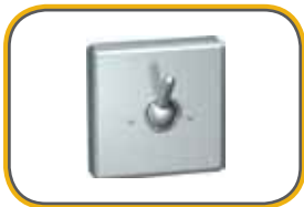
122 - 304 stainless steel alloy rear mounted security clothes hook with washers, nuts & zinc plated steel studs. Tensioned to release down when overloaded beyond the 35 lb (16 kg) limit
