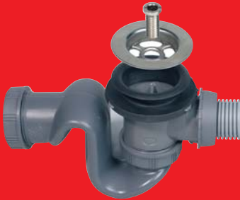
The auto-centring waste washer ensures that the waste stays in position when the grate is screwed on.
